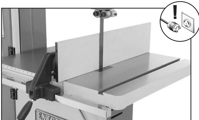
Figure 30. Fence against the blade.
